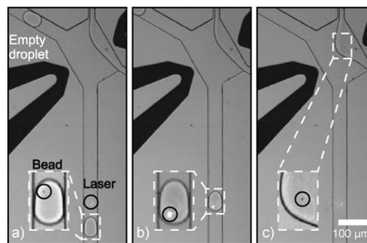
**Figure 4.** Micrographs showing the selection of a droplet containing a fluorescent bead. a) A droplet containing a fluorescent bead approaches the fluorescence detection point. b) As the droplet flows through the laser, the bead emits detectable fluorescence. c) The fluorescence signal triggers an electric pulse which fuses the bead-containing droplet with the lateral stream. The bead can be seen within the lateral stream after the droplet is merged.
