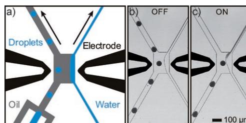
**Figure 1.** a) Scheme of a typical device. Droplets generated on-chip flow parallel to an aqueous stream between two electrodes. b) Micrograph of a typical device in operation in the absence of an electric field. Droplets of a dye flow past the electrode region without interacting with the aqueous stream. c) In the presence of an electric field, droplets coalesce with the lateral aqueous stream as they enter the electrode region.
