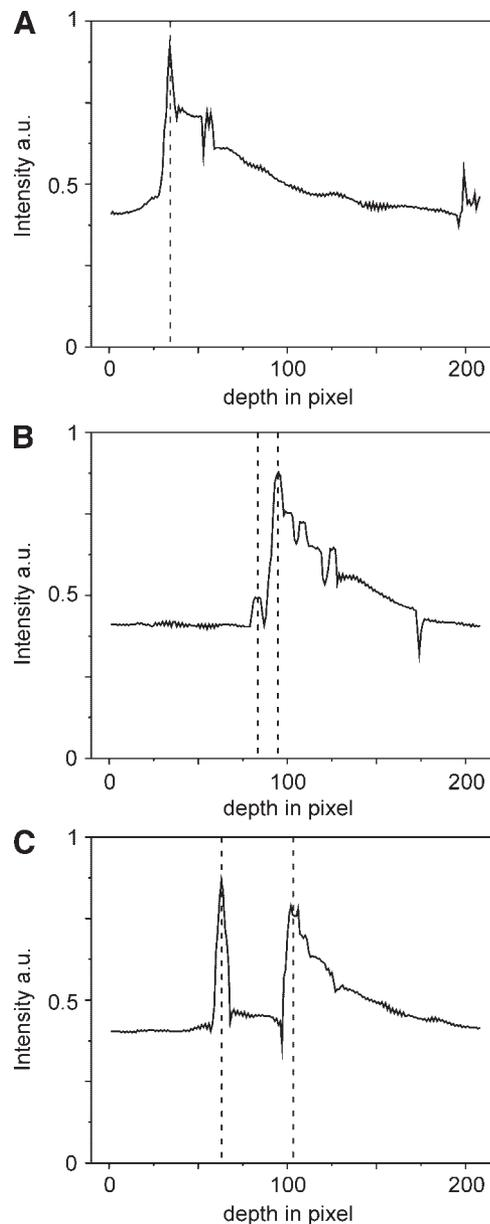
**Figure 3.** Representative cross-sectional depth (B-scan) OCT scans taken from the images in Figure 2. (A) Uncoated tablet A. (B) Tablet B with a single cosmetic coating. The first peak is small compared to the second peak. (C) Tablet C cosmetic and enteric coatings. (D) Complex tablet with three coatings. The dotted lines mark the characteristic peaks that were used for the coating thickness analysis.
