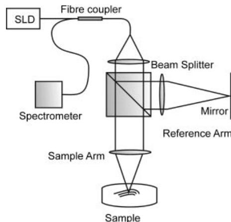
**Figure 1.** Schematic setup of the fibre-based OCT system. The light source is a super luminescent diode that has a large spectral bandwidth. After travelling through the beam splitter, the light scattered back from the sample is superimposed on the reference beam and travels back to the fibre coupler to give an interference pattern in the spectrometer, which is evaluated after Fourier transformation.
