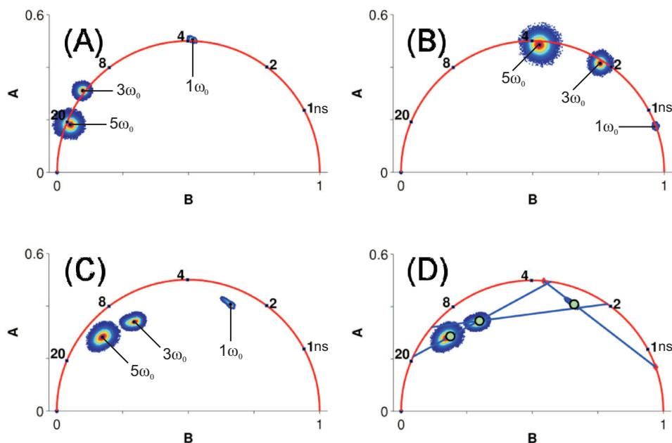
Fig. 6. Phasor plots from mhFLIM measurements at  $1\nu_0$ ,  $3\nu_0$ , and  $5\nu_0$  for (A) Rhodamine 6G in ethanol. (B) Rose Bengal in ethanol. (C) Rhodamine 6G and Rose Bengal mixture in ethanol. (D) The same dye mixture shown with a biexponential estimate from Eq. (6). The numbers along the semicircle indicate the single-exponential lifetimes for measurements at the fundamental frequency.
