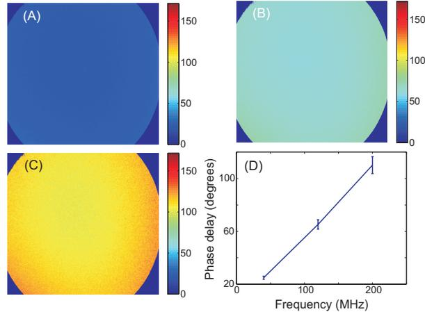
Fig. 5. Phase variation across the ICCD at the fundamental frequency of  $\nu_0 = 40$  MHz (A), the third harmonic of  $3\nu_0 = 120$  MHz (B) and the  $5\nu_0 = 200$  MHz. (D) The mean phase delay versus frequency; error bars indicate the standard deviation. The data were obtained from a calibration with Rose Bengal dye.
